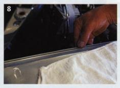
off the distributor shield to gain access to the coil wire, which would come in handy later during the cranking-compression check. While he was in there, he inspected the wires and contacts for cracking, corrosion, and condition.
