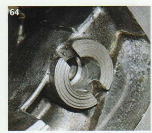
tered over the shiny dimple in the side of the case near the gear drive. If it all looks good, pull the cover back off, goop the back of the bearing support with RTV, and stick on the new gasket. With the reverse-shift gear clicked forward, line the reverse-gear pin (photo 63) up with the back of the cover (photo 64) and mate the two halves (photo 65). It may take a little wiggling of the reverse arm to get everything happily in place.
