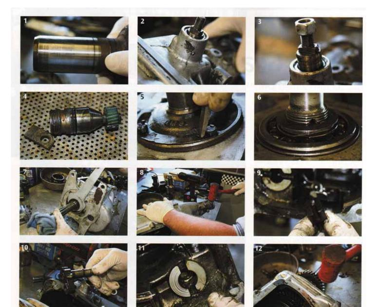
engage any two shift forks with any two gears simultaneously. Then, with the mainshaft effectively locked, take a thin-head gear wrench and loosen the nut by turning "backward," ie. clockwise (photo 7). When it's loose, move the forks back and disengage the gears. Take out the side-cover bolts and the whole assembly will pop off, leaving the shift forks and two shift cams sticking out of the cover.
