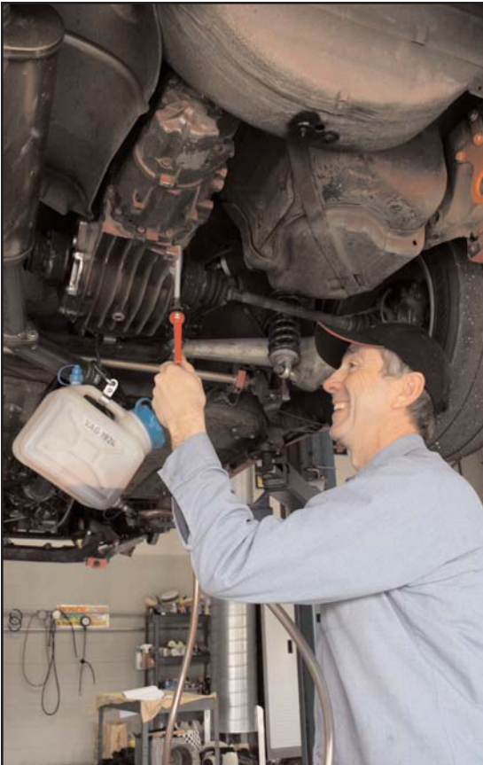
left:and above: Tony pumps fluid into the transmission with a special heated Porsche pump and nozzle.
