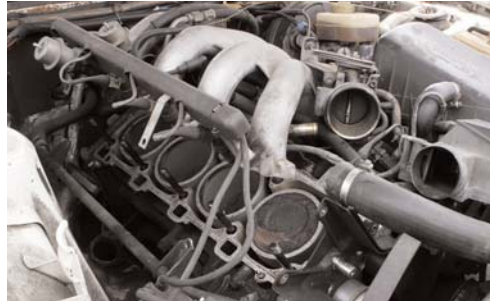
above: This 944 lost its timing belt. above right: The head must be removed. below: Here's the timing belt - the teeth simply sheered off.
