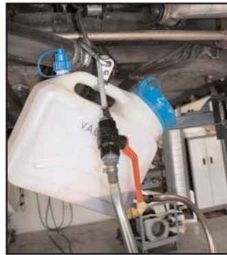
left:and above: Tony pumps fluid into the transmission with a special heated Porsche pump and nozzle.
