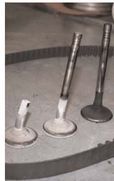
above left: A bent valve sticking out of the head. above center: Removing the valves. above right: Broken, bent, and straight valves.
