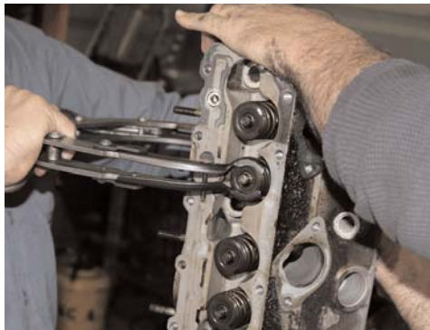
above left: A bent valve sticking out of the head. above center: Removing the valves. above right: Broken, bent, and straight valves.
