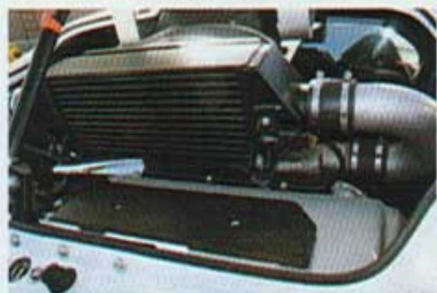
Below: Intercooler is unchanged on S 240, but the model's more efficient scoop feeds it more air.
