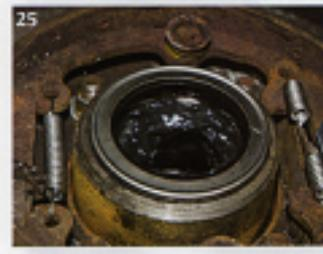
J: After cleaning and inspecting the old spindle-support bearing carrier, mount the arm in a vice and gently tap out the races from behind using the small notches provided (photo 13). Alternate sides, tapping gently to ease the race out without becoming cockeyed.
